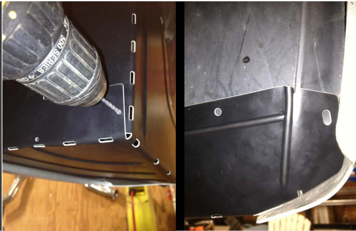
With the box held in place you can now take a 1/8" drill bit and drill ONLY the hole farthest back (shown in left photo) do not install the rivet yet. Some trucks will only line up 2 of the rivet holes. You can push on the back of the box to bring it forward a little to help with lining up the rivet holes .You can also mark the last oval hole on the outside of the air box (Shown on right)
