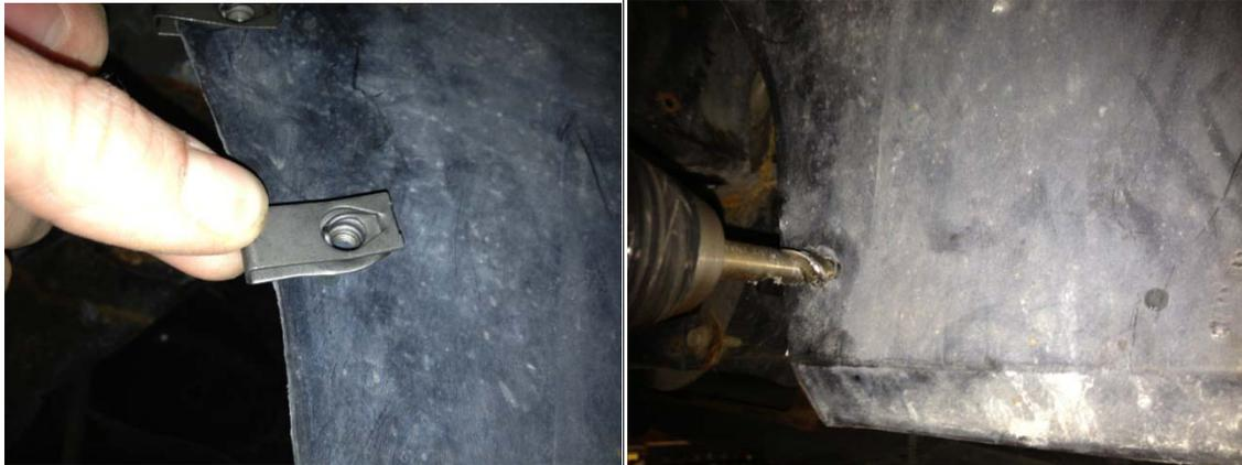
Now remove the air box and make sure the U-Nuts reach the marked hole. If they reach, then using a 3/8" drill bit go ahead and drill the holes. You may want to use a razor blade after to clean up the melted plastic around the holes so the u-nut sits nice and flat.
