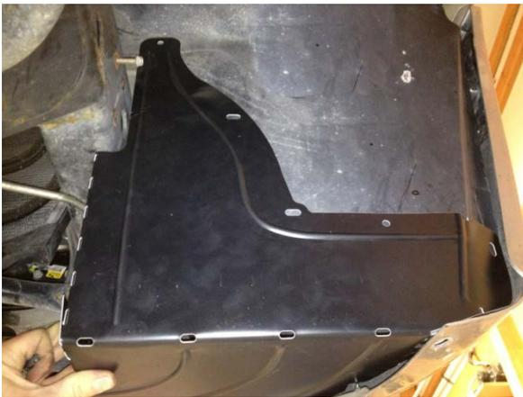
We will now mark the Plastic wheel well liner for some of the holes required to install the supplied “U-Nuts”. You will want to hold the Inside up so that the air box edge is basically parallel to the frame at the
