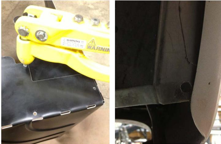
Remove air box and install supplied 1/8" rivet and washer into hole we drilled in the last step. Now drill out the remaining two holes and install rivets with washers on back. Drill the remaining hole you marked in the last step in the plastic wheel well liner with the 3/8" drill bit and install the last U-Nut. (right photo)
