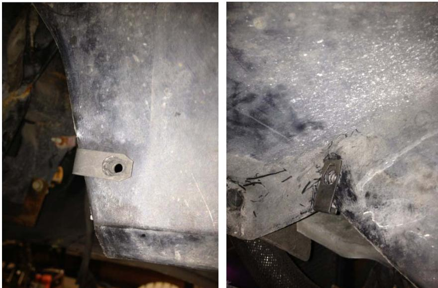
Install U-Nuts onto plastic wheel well liner threaded side facing towards front of truck. (Left picture)
